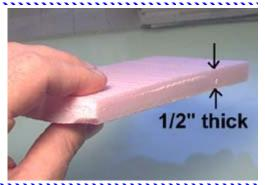
When gluing the blocks down, be sure to spread glue on the **bottom and sides** of the blocks.
