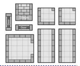
2. We'll start with the **doorway pieces**. Make the floor by gluing **three 1" square floor tiles** down to a piece of mat board.
