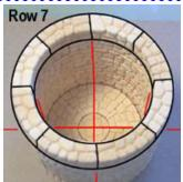
You should **leave the paper ring inserted** while you're stacking and gluing the blocks. At this point you can remove the blocks in the doorway that were used to hold its place.
