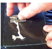
Remove the excess plastic around the side of the mold.
