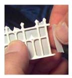
To **remove the excess flash** from the inside of the fence sections, use an x-acto or hobby knife.
