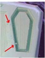
Now for the piece of glass. Be sure to put the **sprayed side of the glass facing down!** If not, plastic will stick to the glass making it difficult to remove the pieces.
