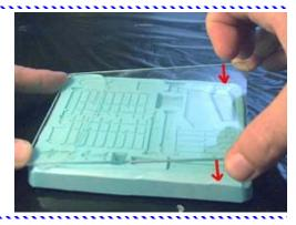
Press down hard on the glass and shove the glass around in a circular motion to remove the excess casting plastic.
